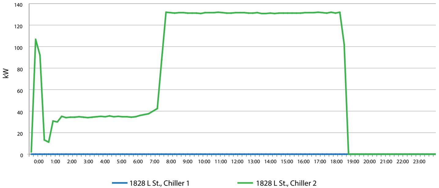
Figure 3: Water Chiller Unit #1 Tripping Offline on May 25, 2012
