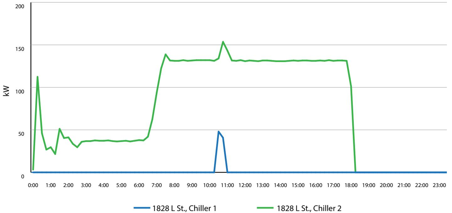
Figure 4: Change in Chiller Nighttime Usage by Correcting Faulty “Optimal Start” Feature
